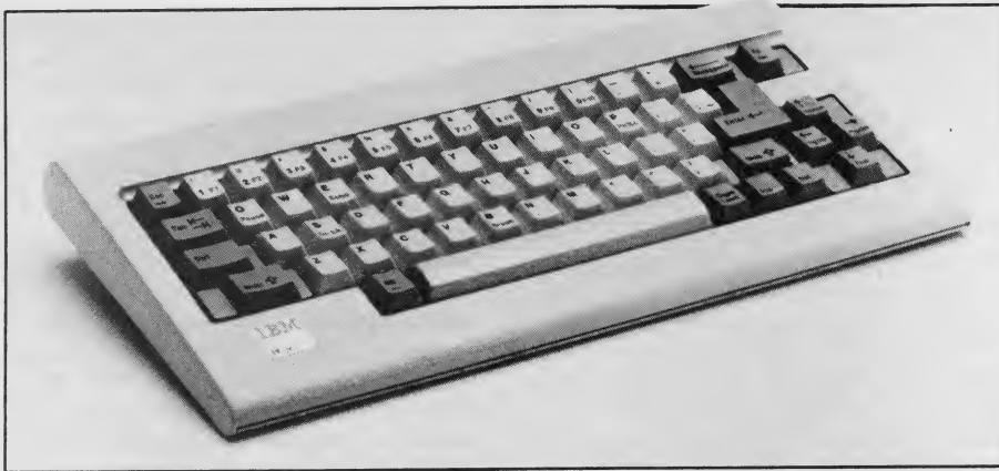
The new IBM PCjr keyboard features 62 full-stroke typewriter style keys in standard QWERTY layout. The built-in infrared serial link has a range of 20 feet.
